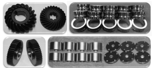
图6 表面沉积了超厚DLC薄膜的齿轮和轴承等异形件照片 Fig. 6 Optical photograph of super thick DLC films on the surface of special-shaped parts such as gear and bearing
